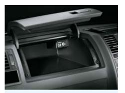
The large glove compartment is lockable. It also contains the front passenger airbag deactivation switch, which can be used when carrying a child seat.
