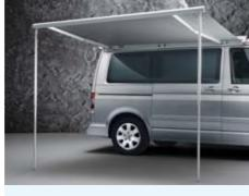
The optional awning is 250cm wide and mounted above the sliding door in the standard attachment channel. The awning case is silvercoloured. For the paint finishes Off-road grey and Shadow blue metallic and Diamond black and Samoa red pearl effect, the case comes in black.
