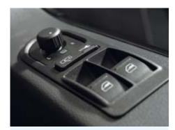
Control unit for electric door mirrors, windows and central locking.
