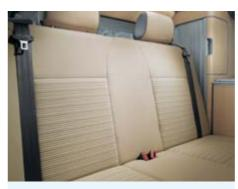
The rear bench/bed slides easily along two rails in the floor. Both seats are fitted with inertia reel seat belts and ISOFIX anchorage points. Folding down the backrest and the padding of the rear luggage compartment cover creates a bed measuring 114 x 200cm.
